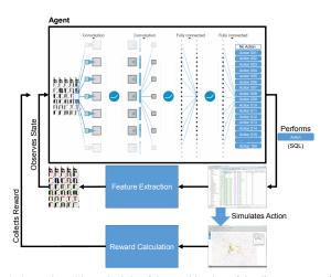
Figure 4: General working principle of the combination of the discrete-event simulation with the DQN algorithm. Convolutional network graphic adopted from [17].
